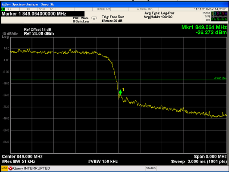
WCDMA band V band edge-right side (HSUPA)
