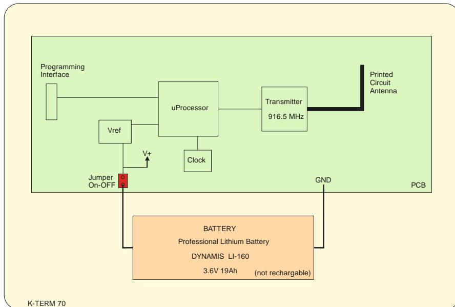
The K-TERM70 electronic is placed in an IP65 case. No external wires or connectors.
