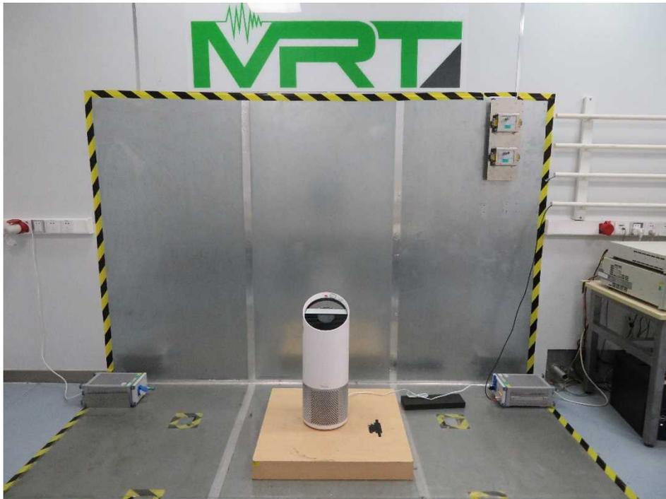
**Field Strength and Harmonics Test Setup**
