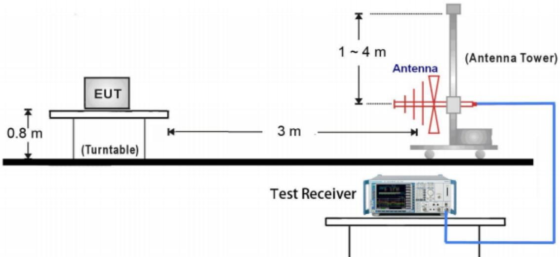
1GHz ~ 18GHz Test Setup:
