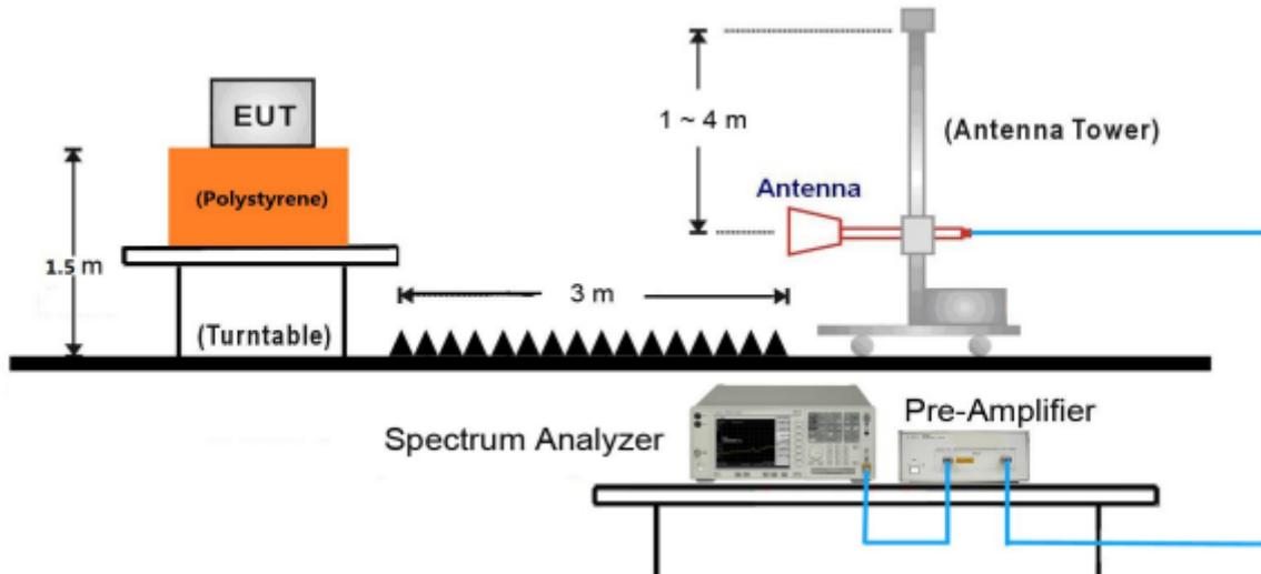
18GHz ~ 25GHz Test Setup:
