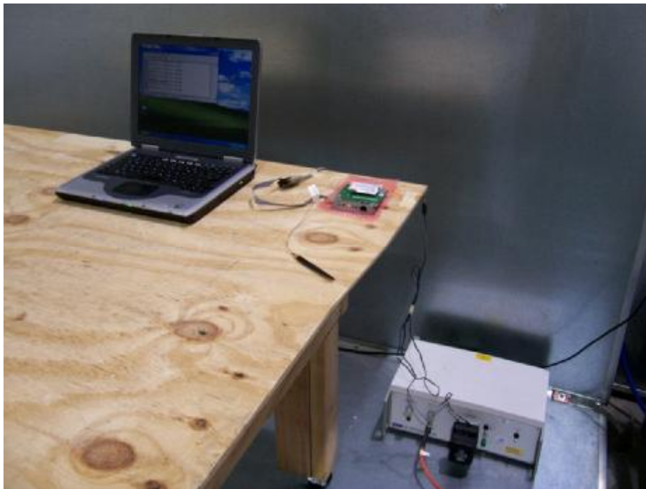
Conducted Emissions Voltage Setup
