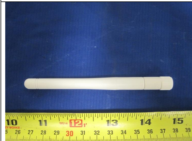
Antenna – Top View (Sleeve antenna)
