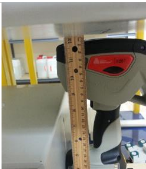
Top Side 5 mm distance from the phantom
