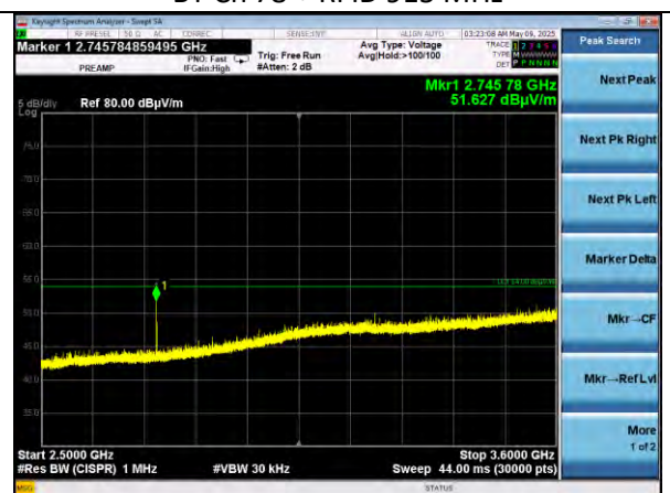
2.5-3.6 GHz Vertical Polarity BT Ch 78 + RFID 915 MHz
