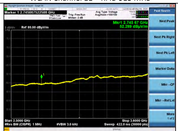
2.5-3.6 GHz Vertical Polarity WLAN Channel 1 + RFID 915 MHz
