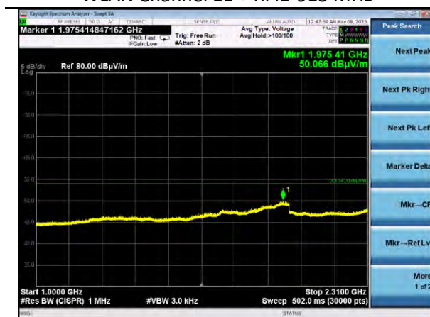
1-2.31 GHz Vertical Polarity WLAN Channel 1 + RFID 915 MHz
