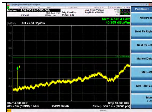
4-18 GHz Horizontal Polarity Tx 915.25 MHz EUT Flat
