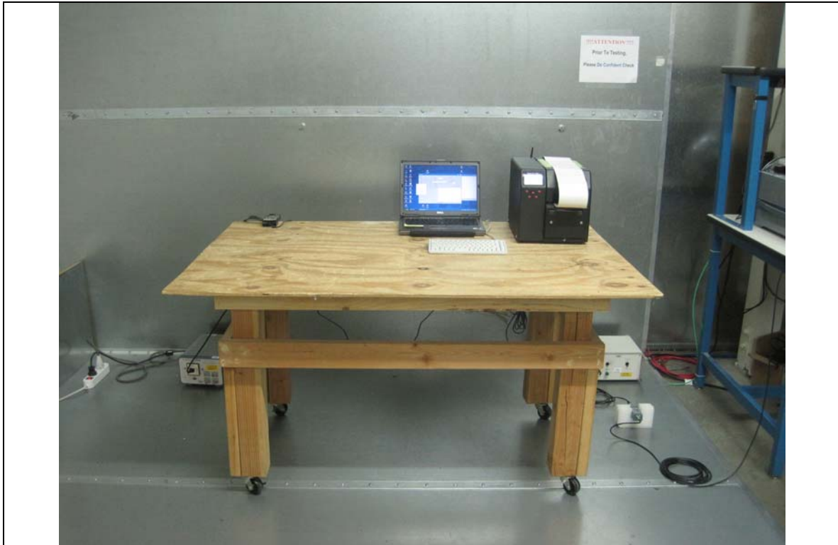
Host: 9906 Conducted Emission Test Setup – Front View
