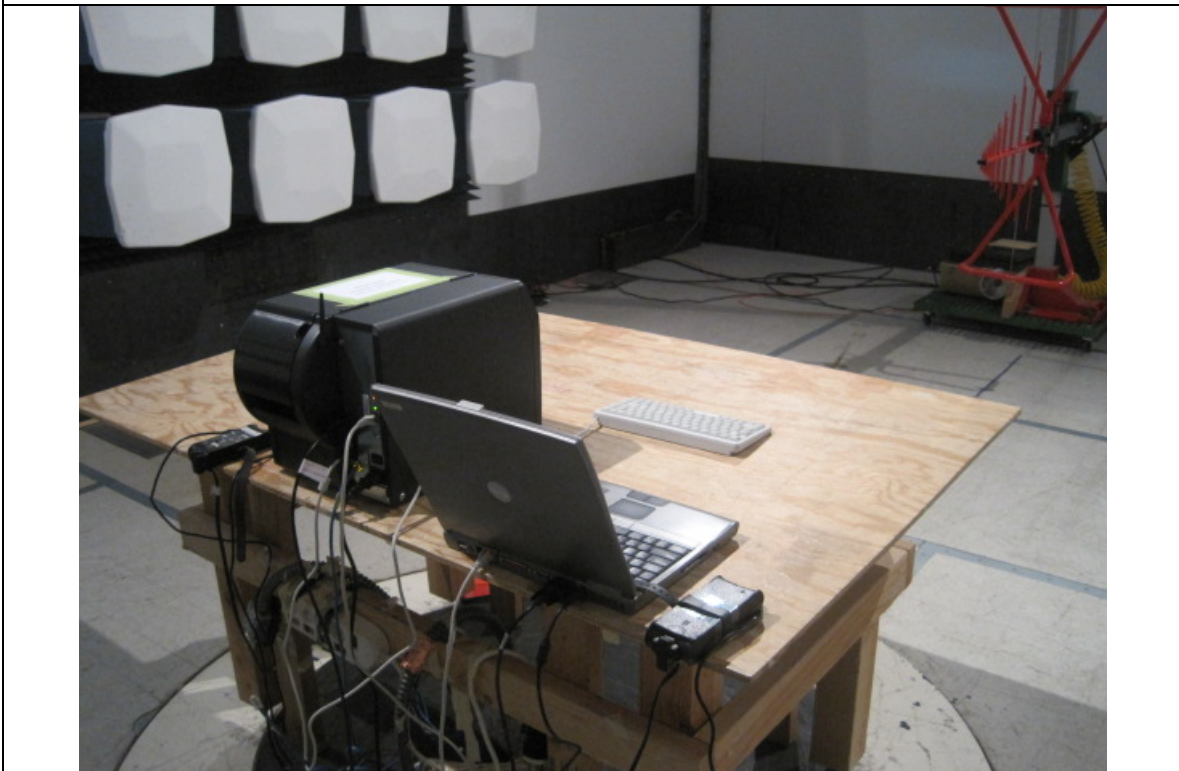
Host: 9906 Radiated Emission Test Setup – Rear View
