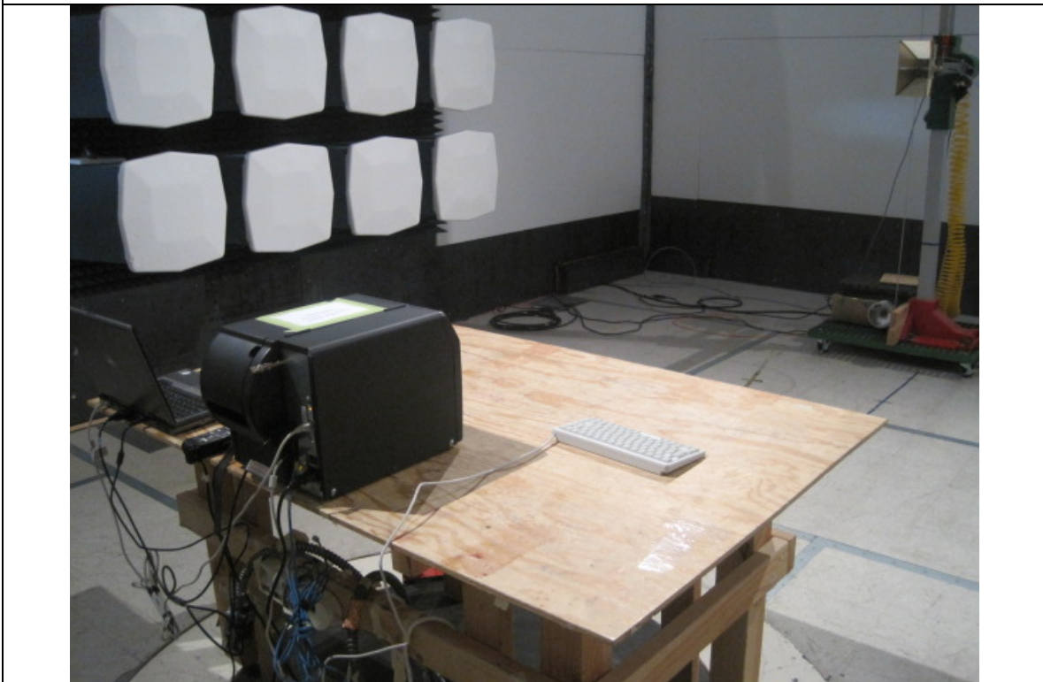
Host: 9906 Radiated Emission Test Setup – Rear View
