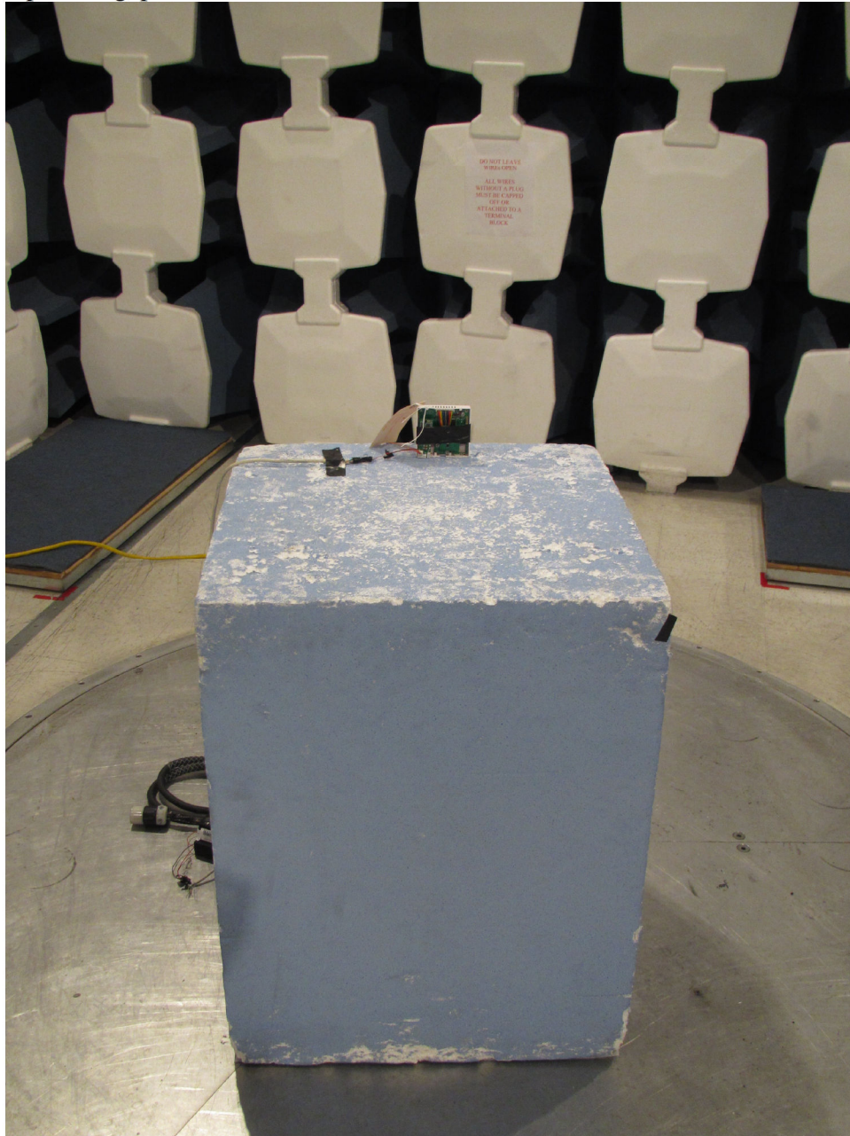
Radiated Emissions – Back
