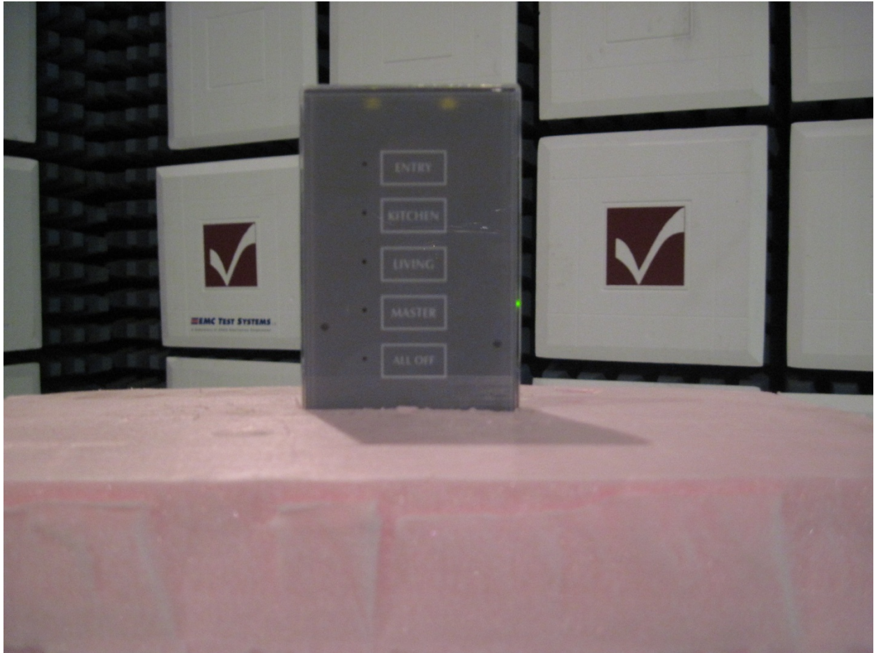
Radiated Emissions Test Setup Photo
