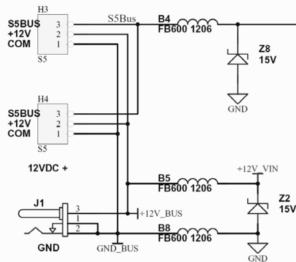
2. S5Bus interface circuit communicates with other devices by bus mode.
