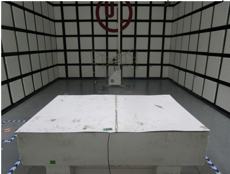
RADIATED RF MEASUREMENT SETUP (Below 30MHz)
