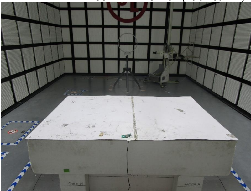
RADIATED RF MEASUREMENT SETUP (Below 30MHz)
