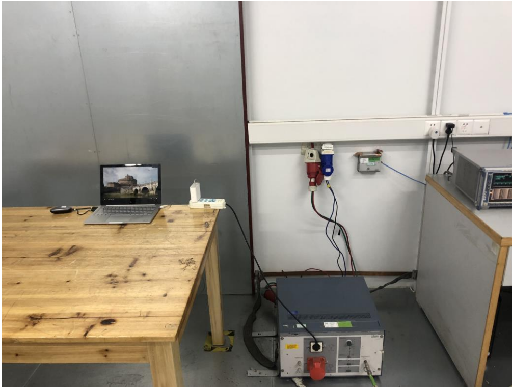
FCC RADIATED EMISSION TEST SETUP BELOW 1GHZ
