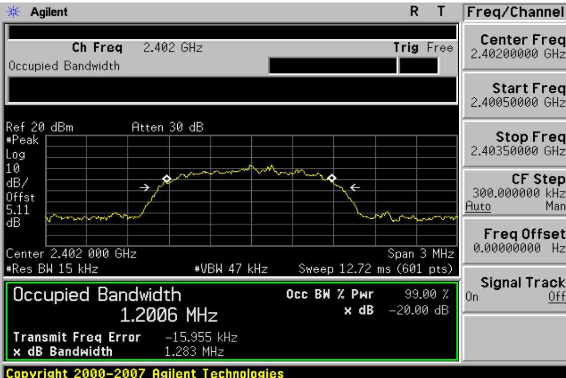
**20dB Bandwidth Test Data CH-Mid**
