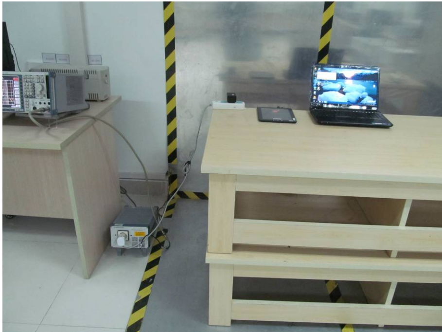
FCC LINE CONDUCTED EMISSION TEST SETUP
