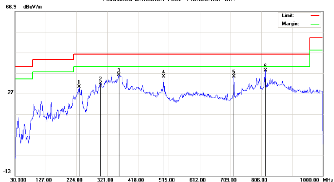
Radiated Emission Test –Horizontal -3m
