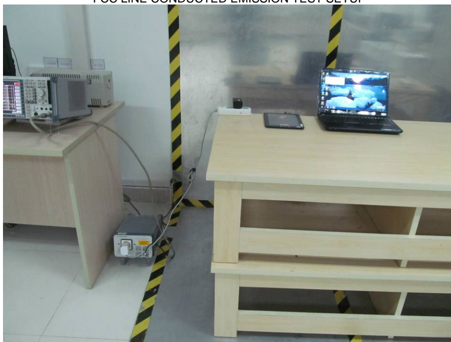
FCC LINE CONDUCTED EMISSION TEST SETUP
