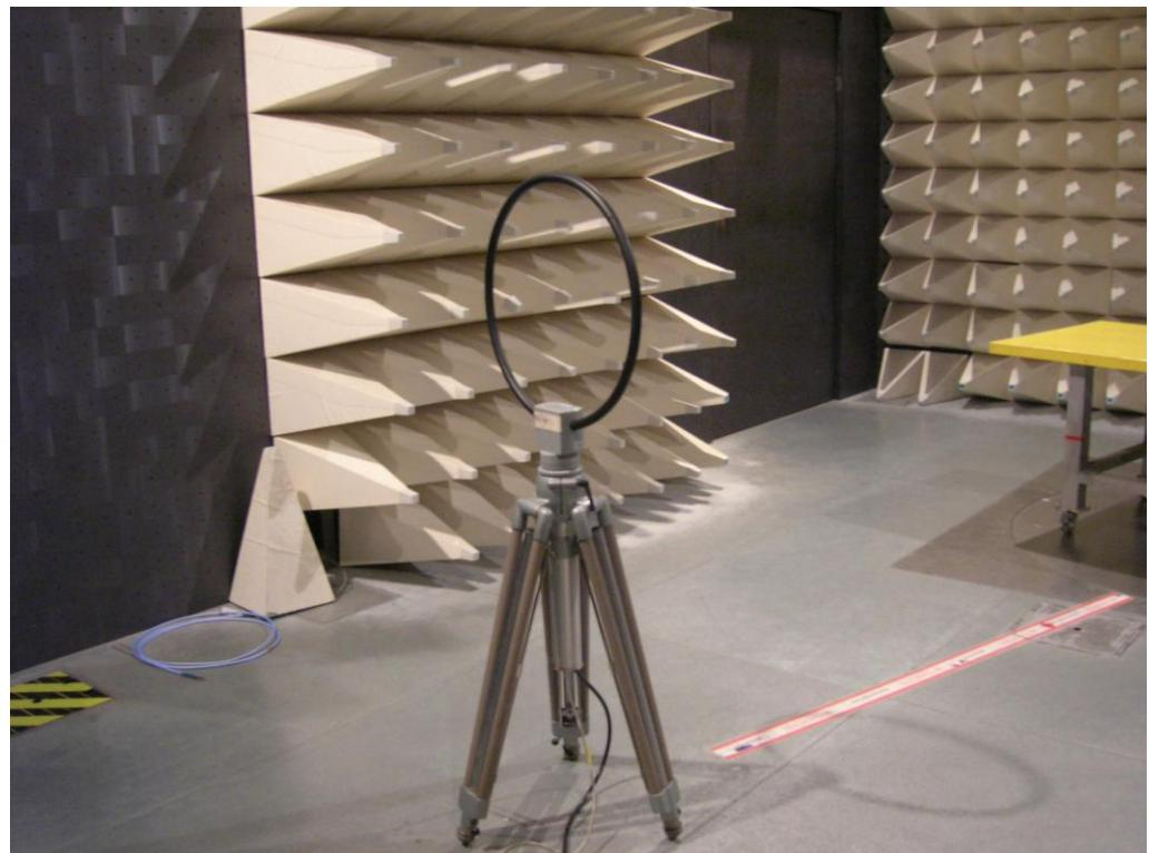
For radiated emissions 30MHz~1GHz
