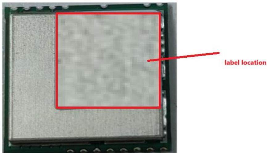
The label is attached to the surface of the shield with a permanent adhesive.
