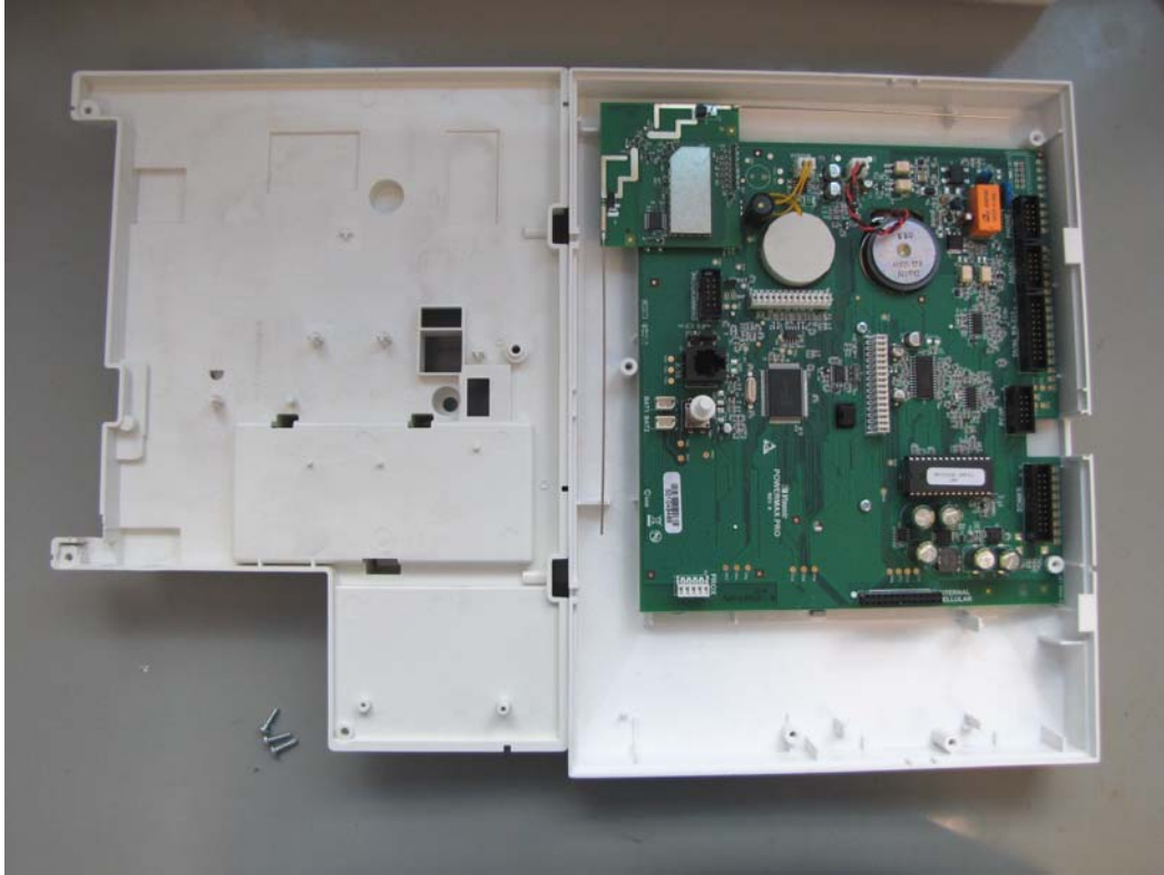
Photograph No.4 PowerMax Pro main part with cover removed view
