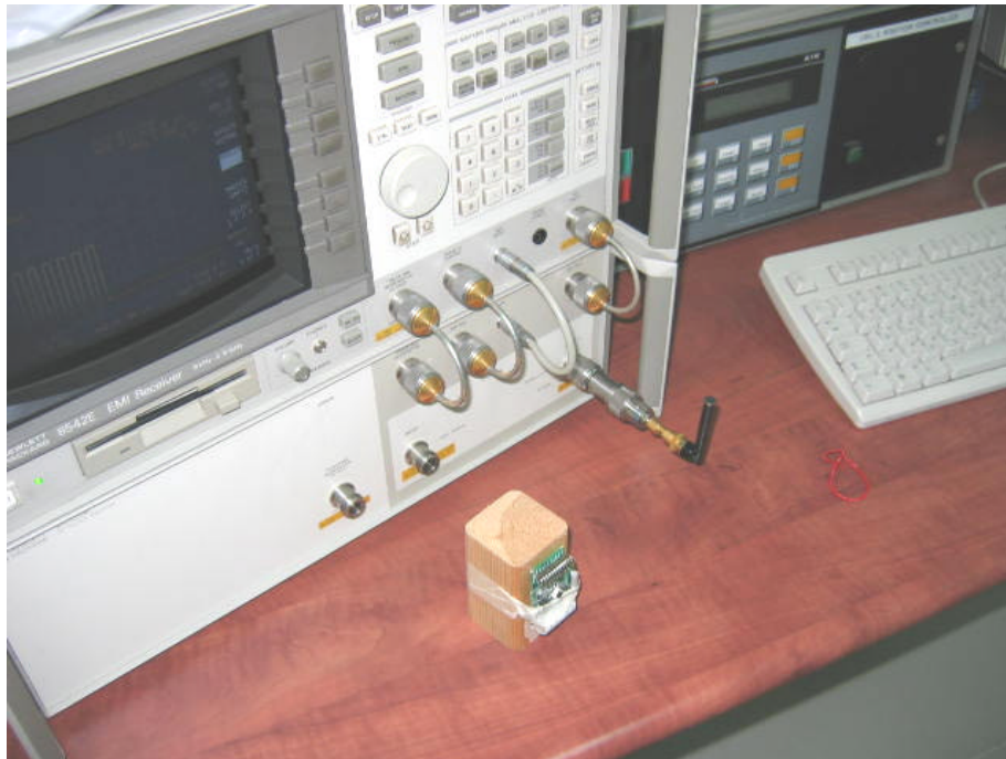
Photograph No.4 Setup for occupied bandwidth test
