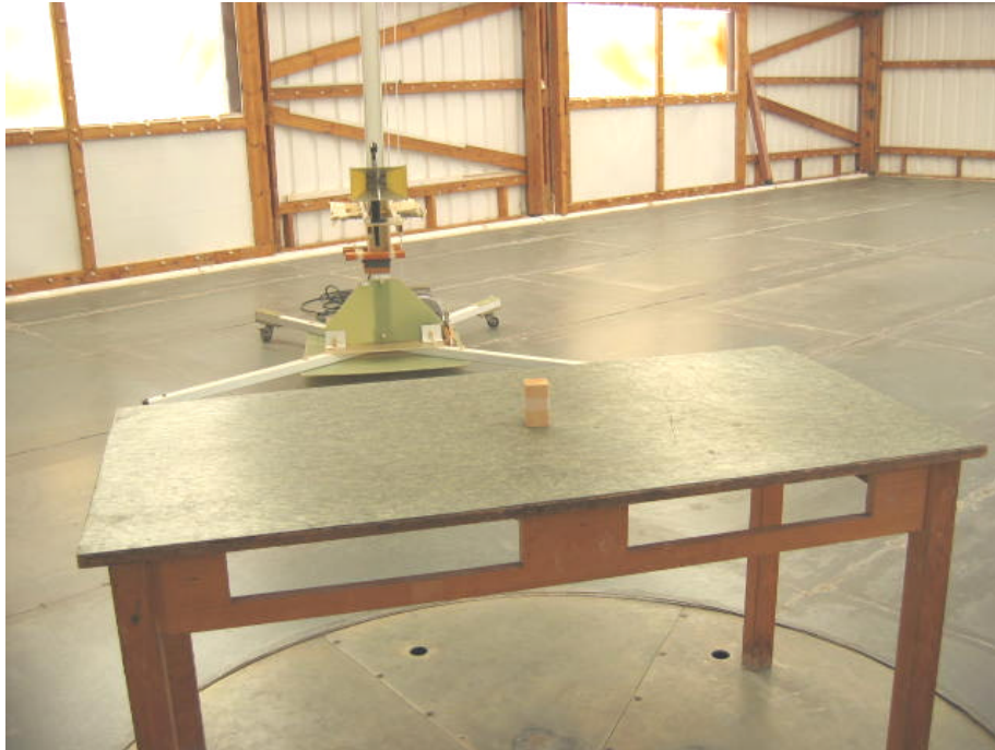
Photograph No.3 Setup for spurious emission field strength measurements at OATS above 1000 MHz
