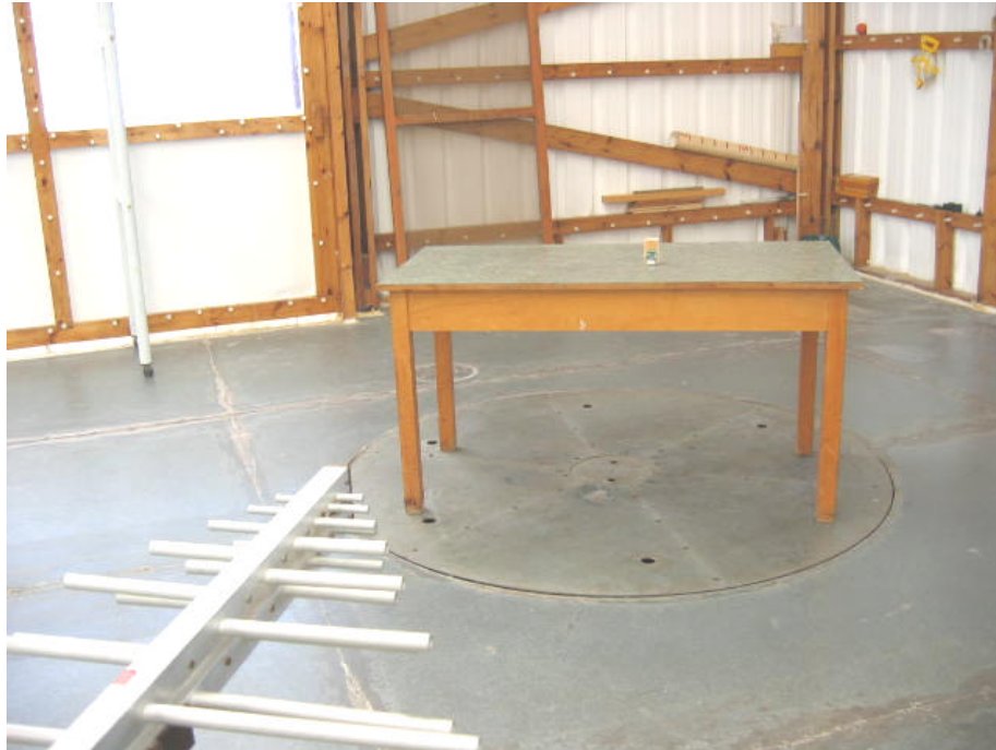
Photograph No.2 Setup for spurious emission field strength measurements at OATS from 30 to 1000 MHz
