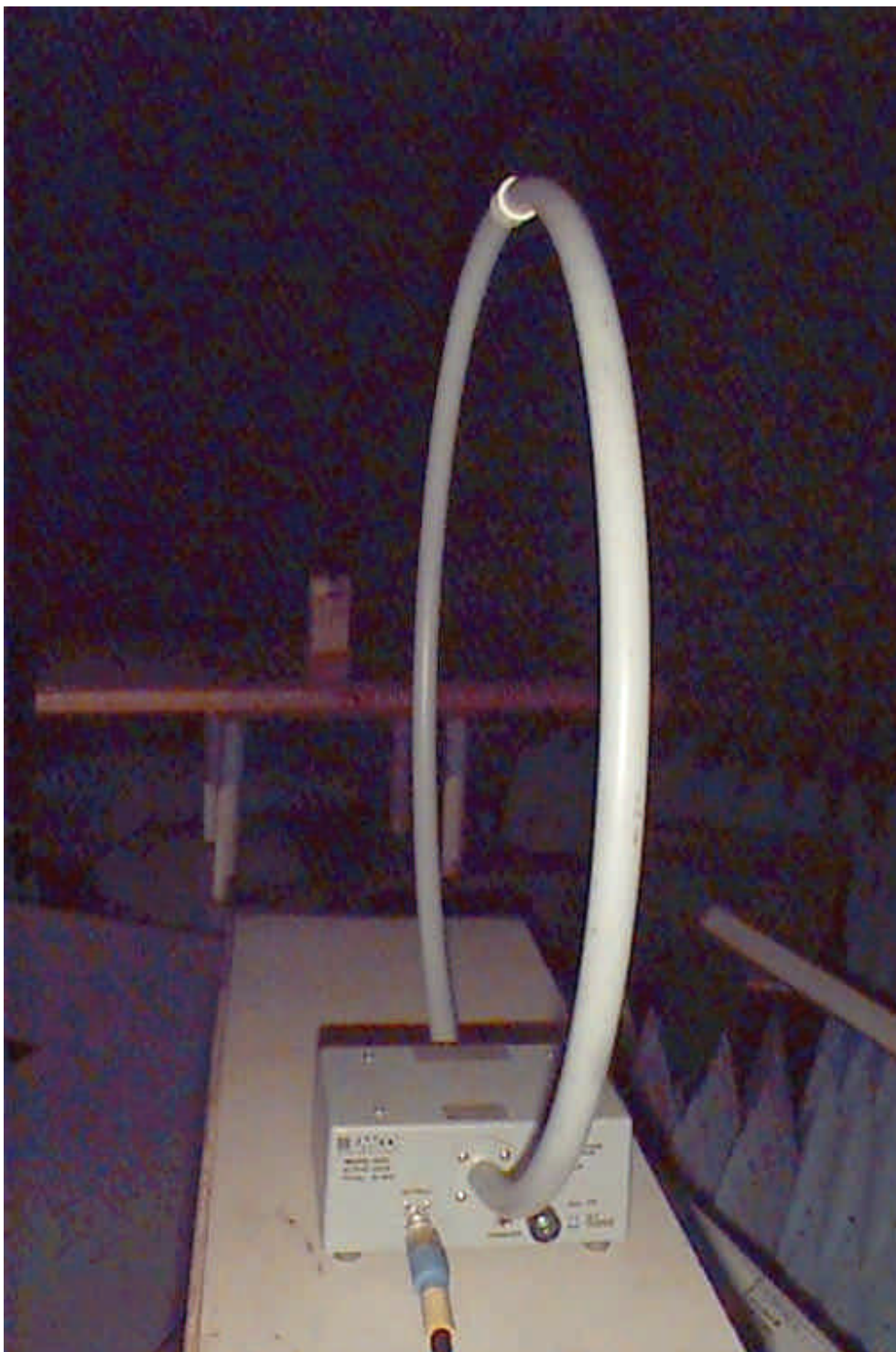
Photograph No.1 Spurious radiated emissions measurement setup in the anechoic chamber with loop antenna
