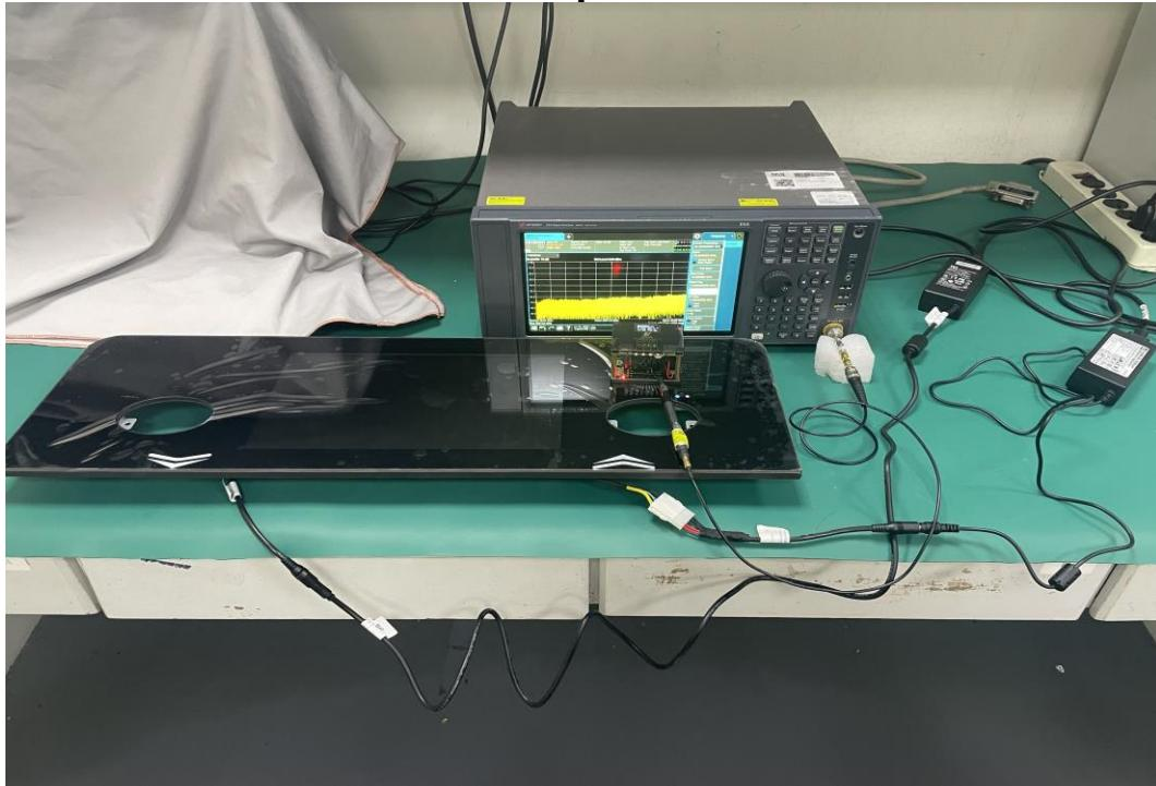
**AC Power Line Conducted Emission Setup Photo**
