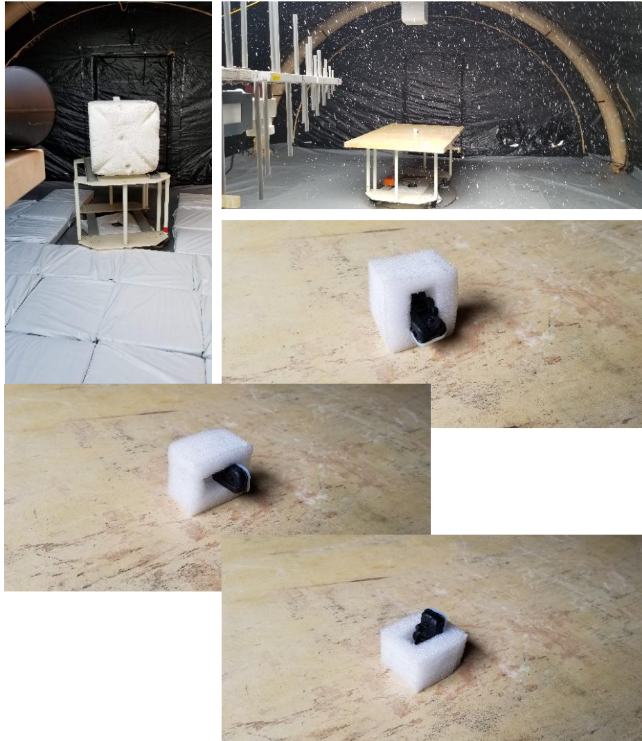
Figure 4: Radiated Emissions Test Setup Photograph(s).
