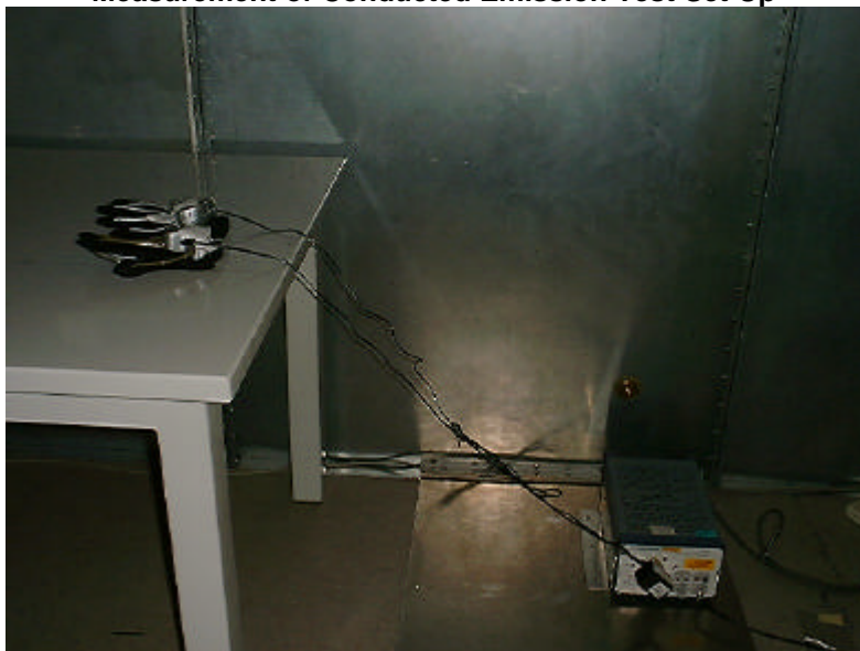
Measurement of Conducted Emission Test Set Up
