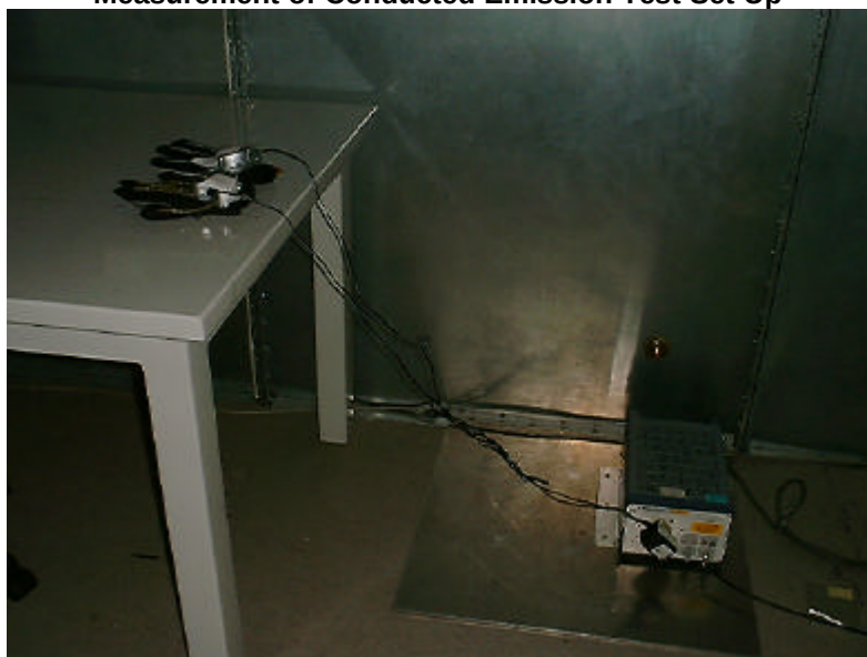
Measurement of Conducted Emission Test Set Up
