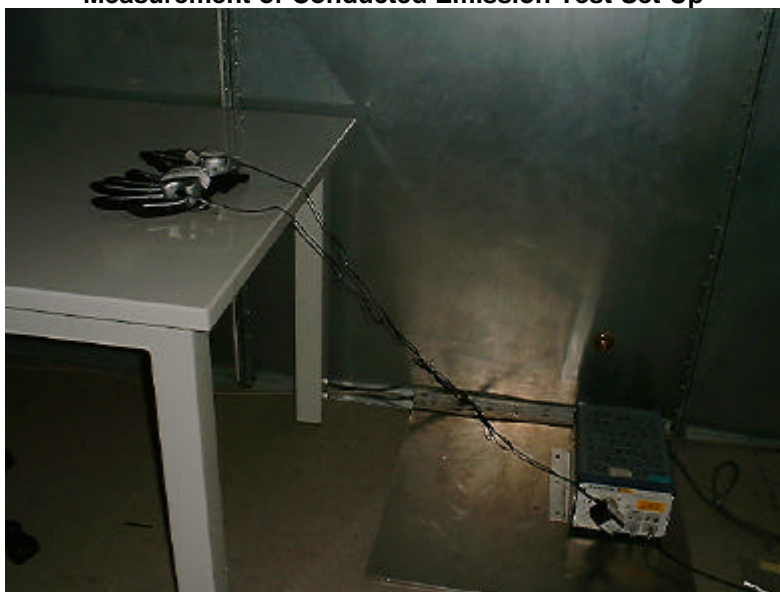
Measurement of Conducted Emission Test Set Up
