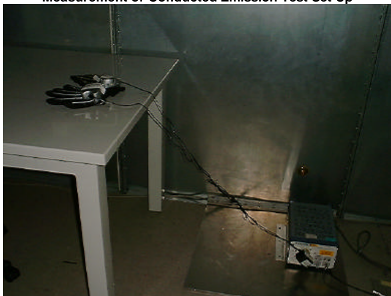
Measurement of Conducted Emission Test Set Up
