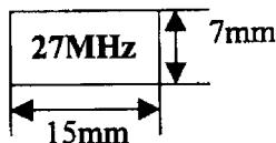
(Remark: Frequency labeling with white print on black and stick on the bottom of TX.
