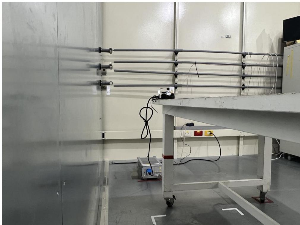
**Radiated emissions test photos****9 KHZ to 30 MHZ**
