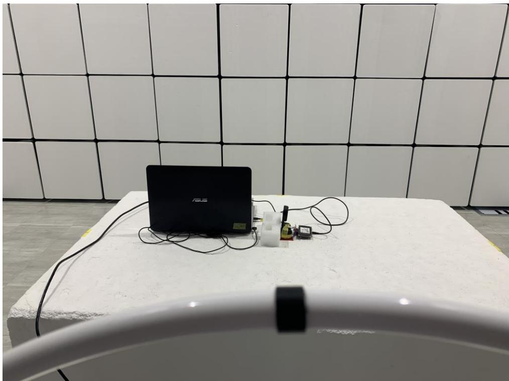
**Radiated emissions test photos****30 MHz to 1 GHz**
