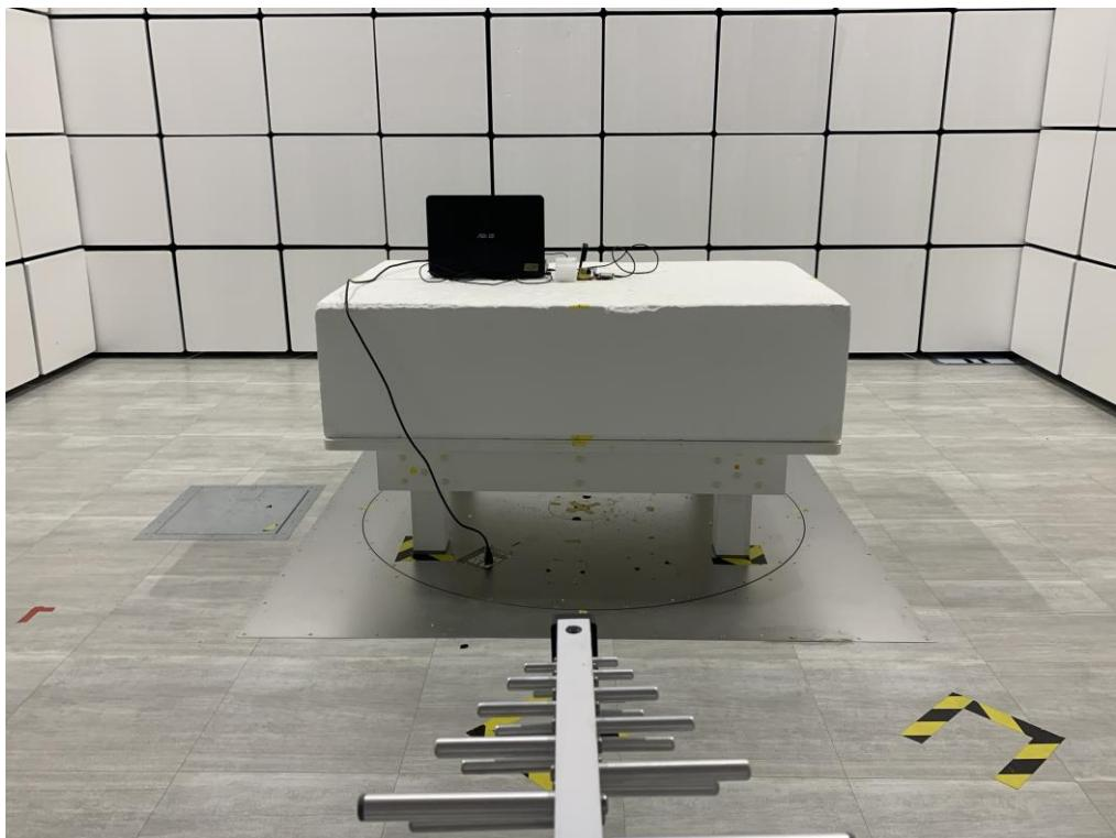
**Radiated emissions test photos****Above 1 GHz**
