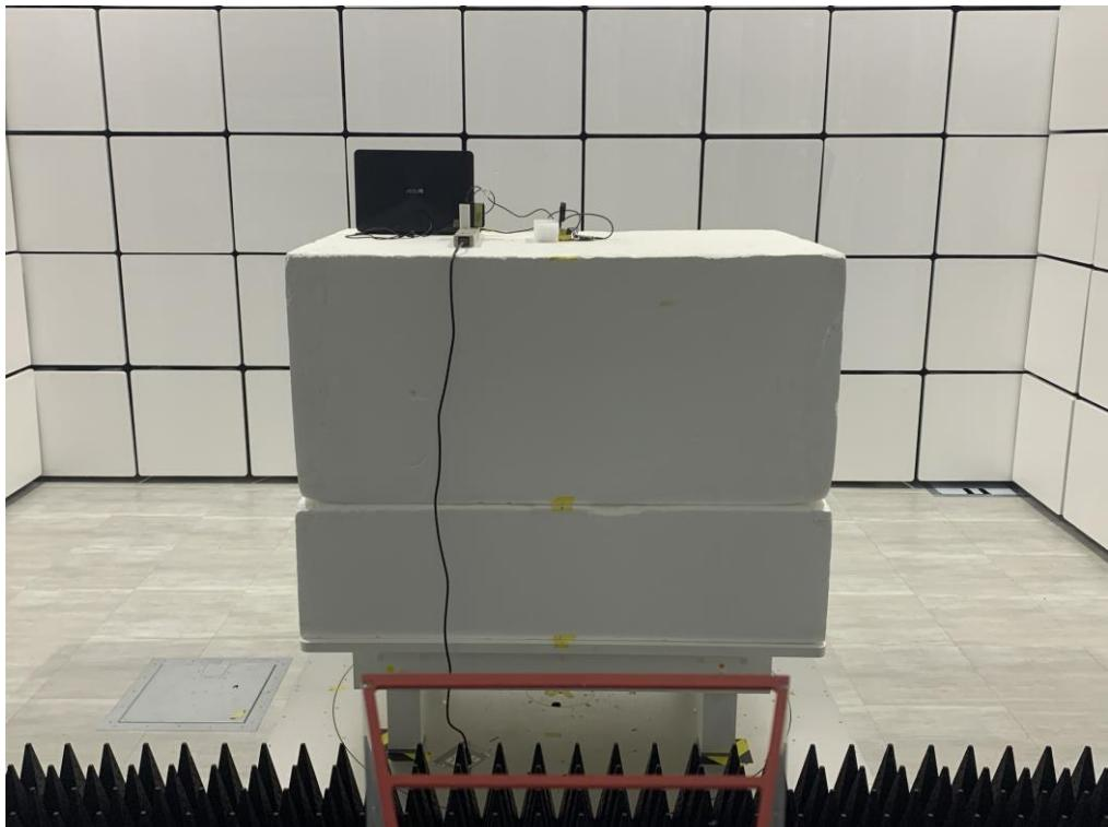
**Radiated emissions test photos****Above 18 GHz**
