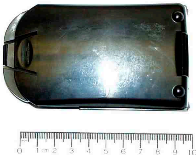
< Rechargeable Li-Ion battery pack, P/N: 1030070, 7.4 V, 1800 mAh >
