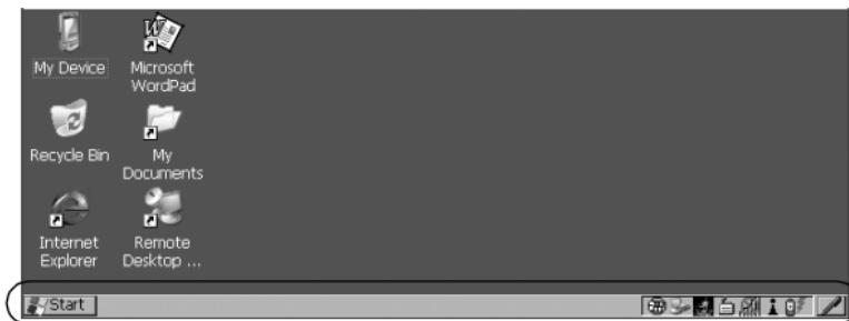
The 8525 G2/8530 G2 has a taskbar at the bottom of the screen. It displays icons through which you can view the internal battery capacity, the radio signal quality of your unit, and so on. If the vehicle-mount is attached to a peripheral device, an associated icon is displayed. In addition, the taskbar displays the application(s) currently running on your unit and the security level assigned to your 8525 G2/8530 G2.
