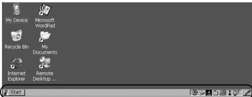
The taskbar changes dynamically, and only those icons that are applicable are displayed. For example, if a radio is not installed in your unit, the radio signal icon is not displayed in the taskbar.
