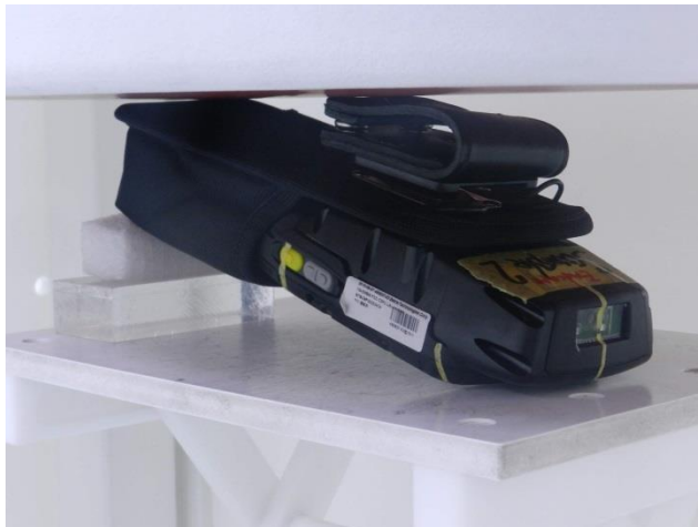
Back with Holster(ST6091), Test Separation 0 cm
