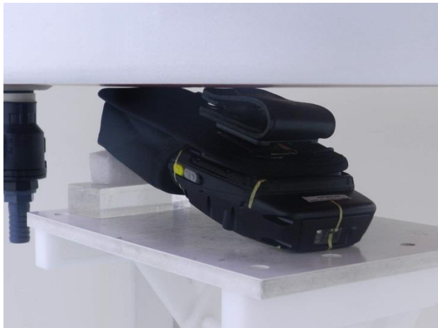
Front with Holster(ST6091), Test Separation 0 cm
