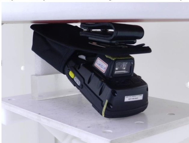
Back with Holster(ST6091), Test Separation 0 cm
