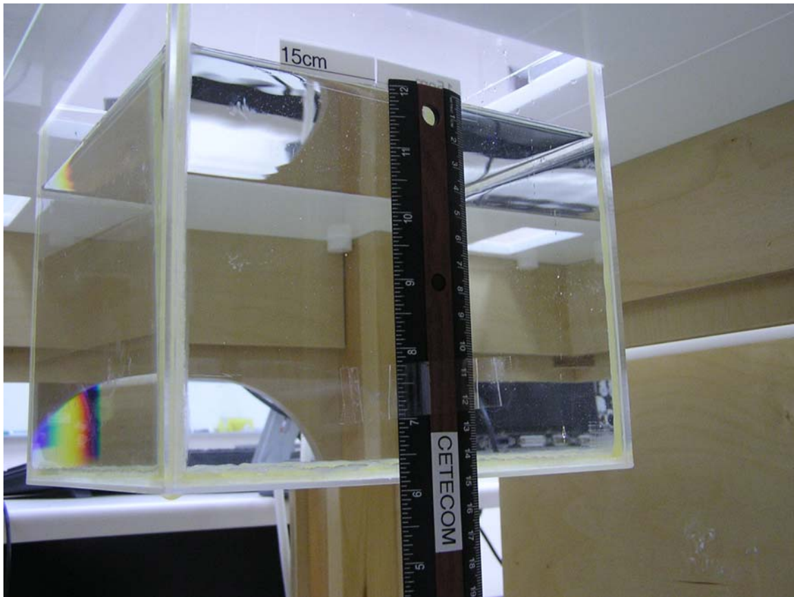
Photo 2. Photo to demonstrate 15 cm Z-axis flat phantom
