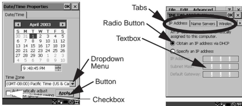
**Note:** Tap the stylus on a dialogue box element to select or deselect it, display a dropdown menu and so on. To use the keyboard, refer to “[Navigating Using The Keyboard](#)” on page 19.
