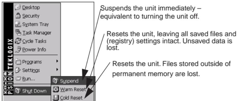
**Note:** This menu varies depending on the security level. At **User** level, the Shutdown sub-menu is replaced with a single option – Suspend. A sub-menu is not available.
