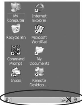
The taskbar changes dynamically, and only those icons that are applicable are displayed. For example, if a Bluetooth radio is not installed, this icon is not displayed in the taskbar. Double-tapping on an icon displays the associated dialogue box.
