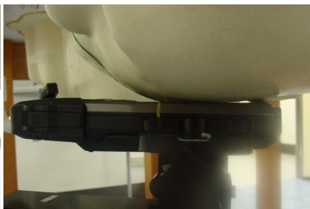
Left Cheek (DUT with Charger Snap Module 2)
