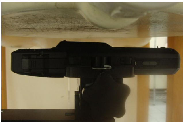
Rear Face of the DUT with Phantom 1.5 cm Gap (DUT with Charger Snap Module 2)
