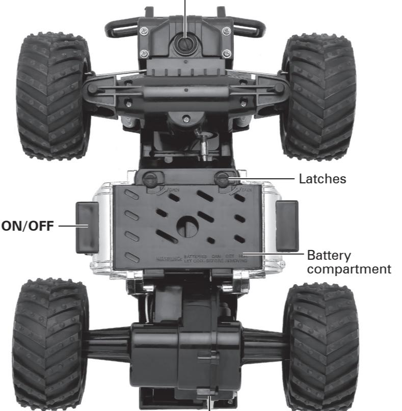
**L / H** – Switch to **L** when driving on rough terrain, or to **H** when driving on smooth terrain.
