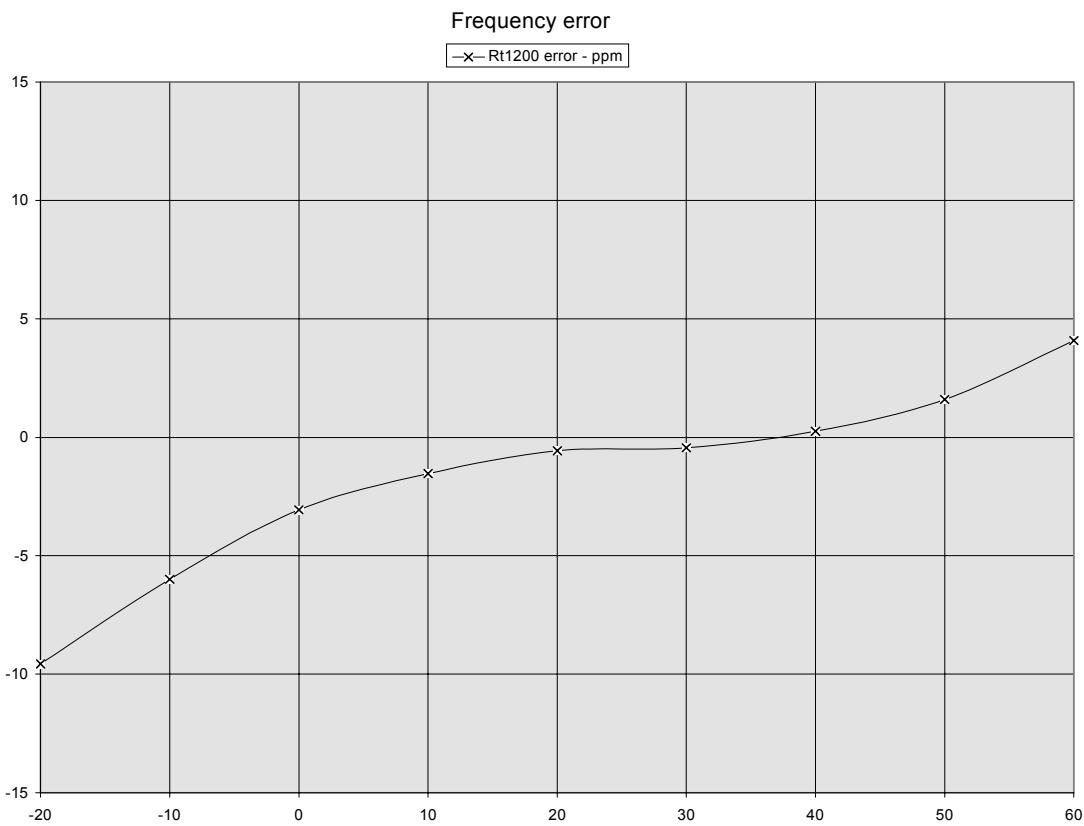
The Transmitter frequency tolerance meets the requirements of Part 80.209(a)
