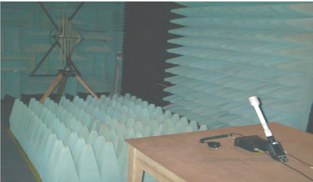
PHOTOGRAPH 5 Layout view of RT1800 during radiated immunity test
