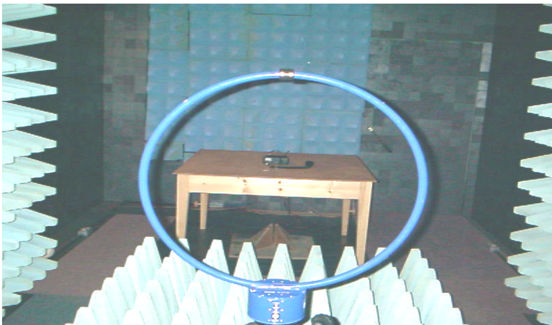
PHOTOGRAPH 1 Layout view of RT1800 during radiated emissions test (150kHz - 30Mhz)
