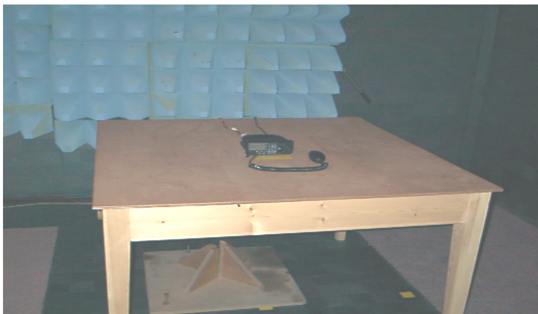
PHOTOGRAPH 2 Close up view of RT1800 during radiated emissions test
