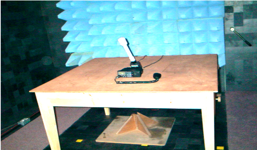
PHOTOGRAPH 4 Close up view of RT1800 during radiated immunity test
