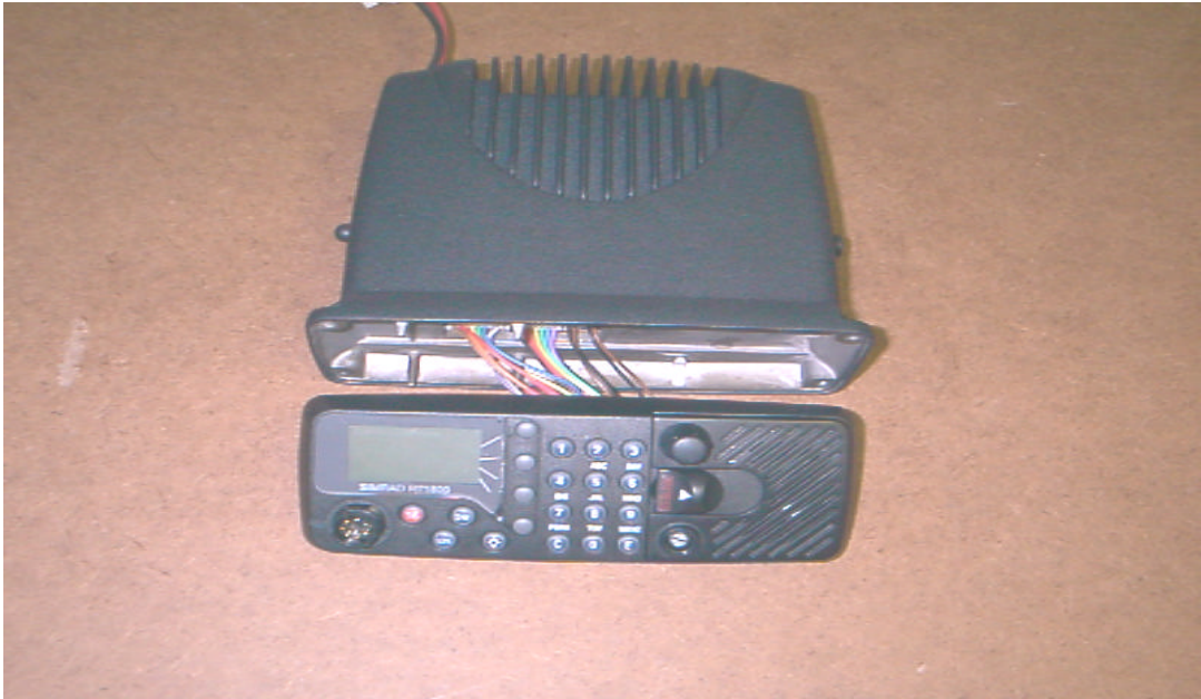
PHOTOGRAPH 12 RT1800 showing the Rx/Tx & front panel sections
