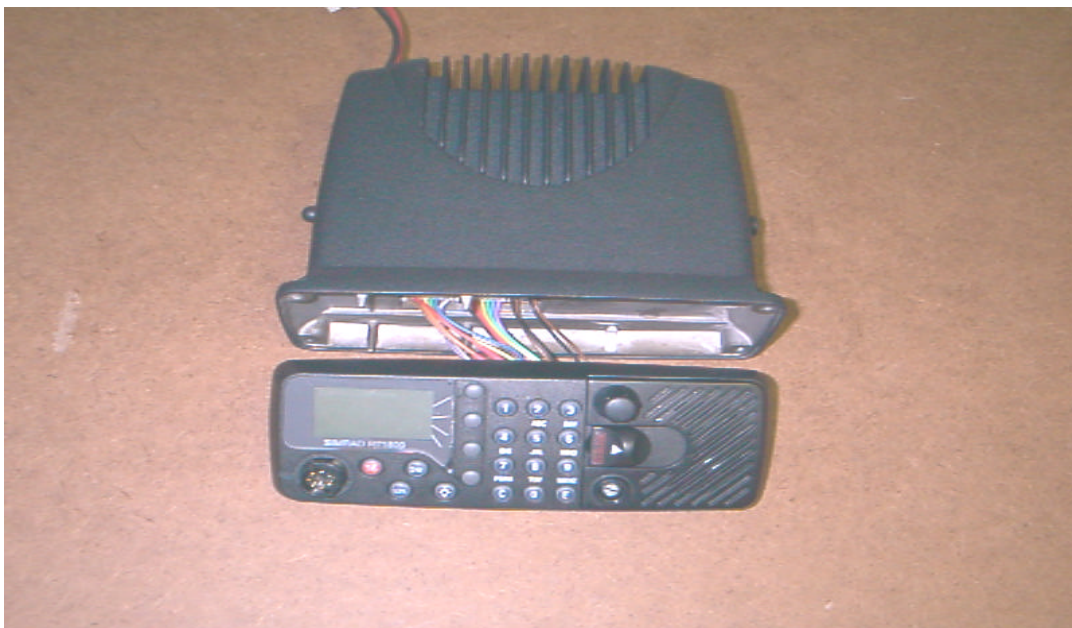
PHOTOGRAPH 5 RD68 showing the Rx/Tx & front panel sections
