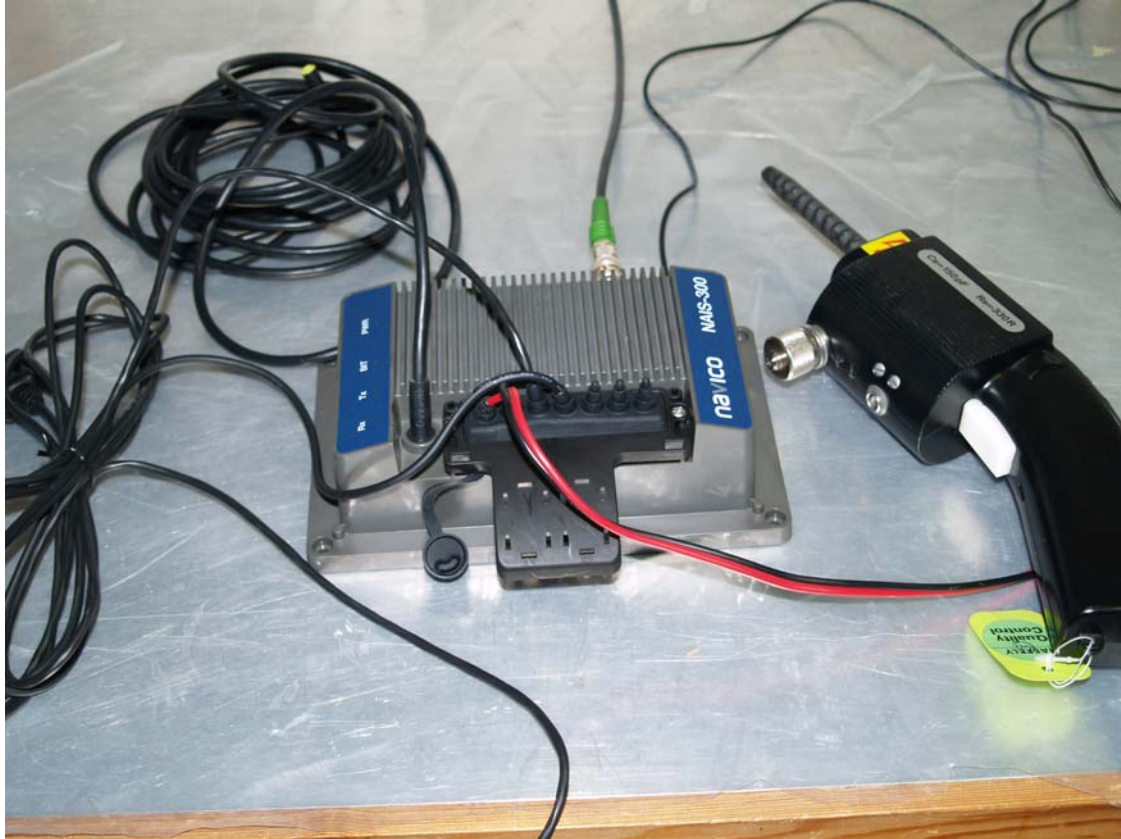
Figure B4.1: Front of EUT showing position of test discharges
