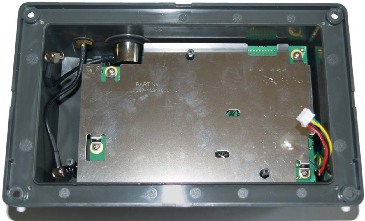
Figure 5: Internal view with top shield and OEM PCB removed.
