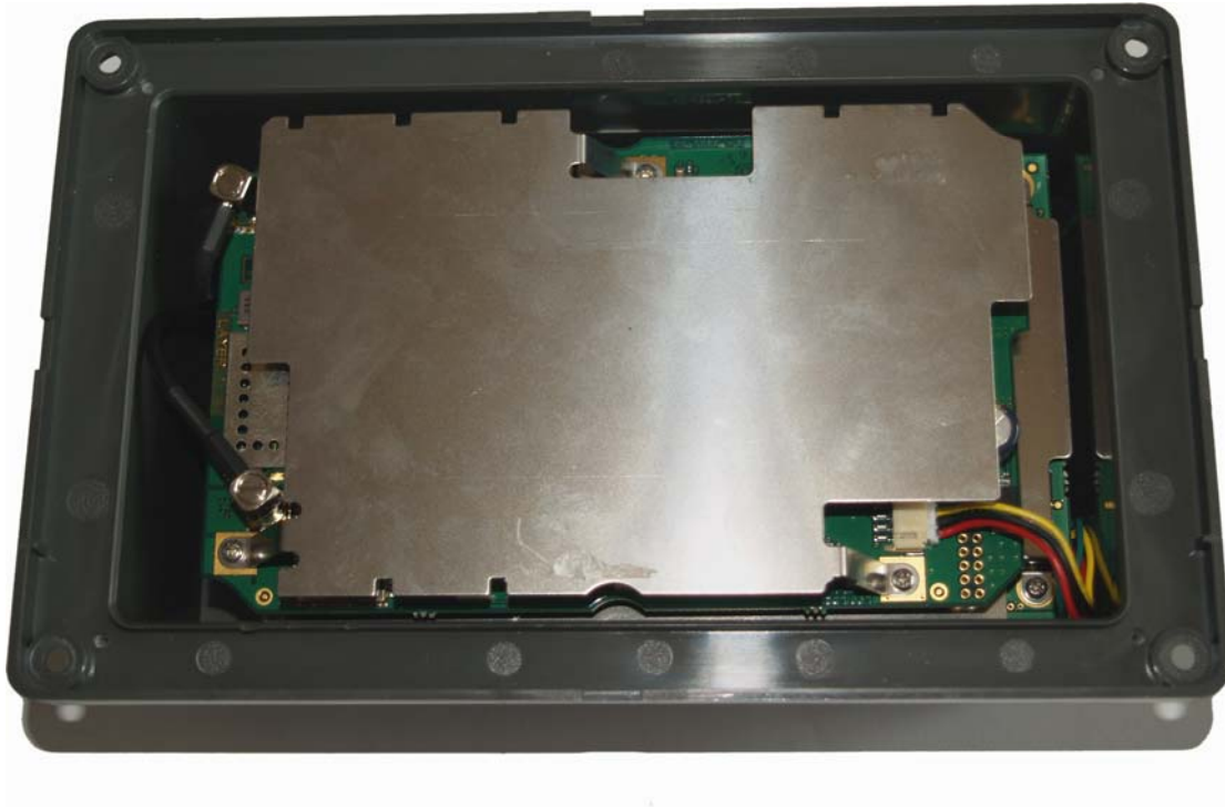
Figure 1: Internal view of NAIS-300 Showing top screen above OEM PCB
