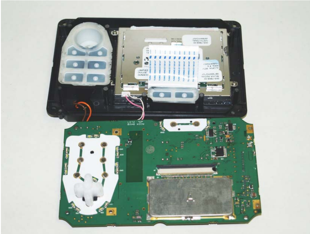
Figure 8: Control PCB in conjunction with LCD and front panel.
