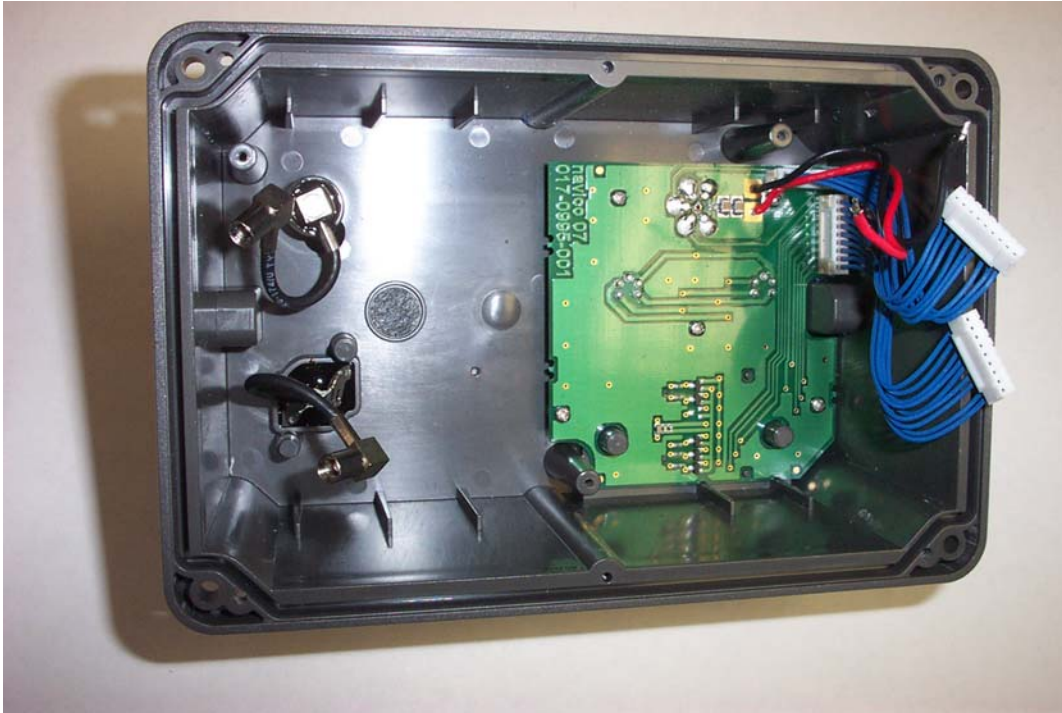
Figure 10: Interior of rear case showing external connector PCB
