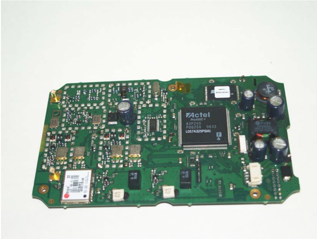
Figure 3: RF PCB FPGA side with screens removed
