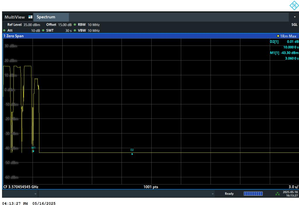
**[Step 5] Configure SAS granted CBSD to operate at frequency 3670-3690 MHz & power level 30 dBm/MHz**
