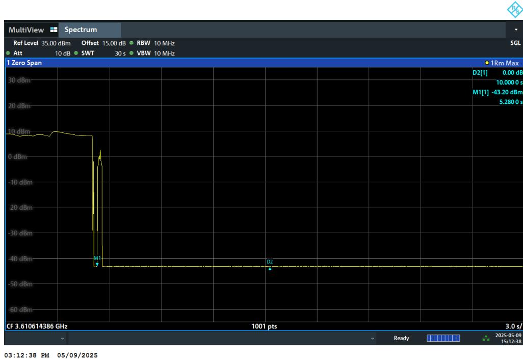
**[Step 5] Configure SAS granted CBSD to operate at frequency 3670-3690 MHz & power level 20 dBm/MHz**
