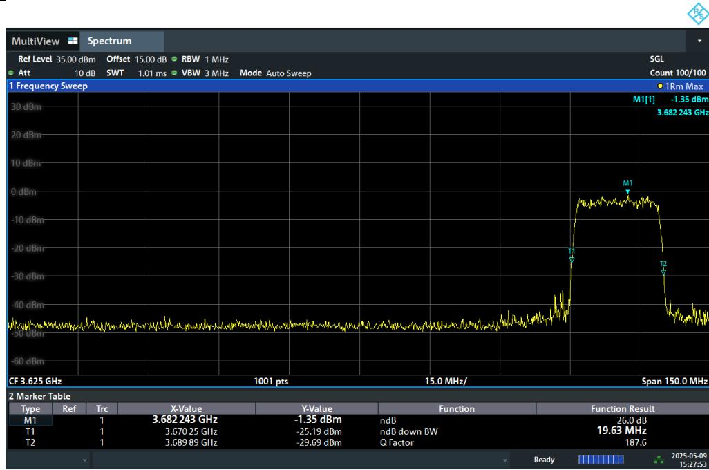
**[Step 8.a.] After changing the frequency and power level, The EUD discontinues operating, changes frequencies, or changes its operational power level within 10 seconds right after receiving instructions from its associated CBSD. Test result is a PASS.**
