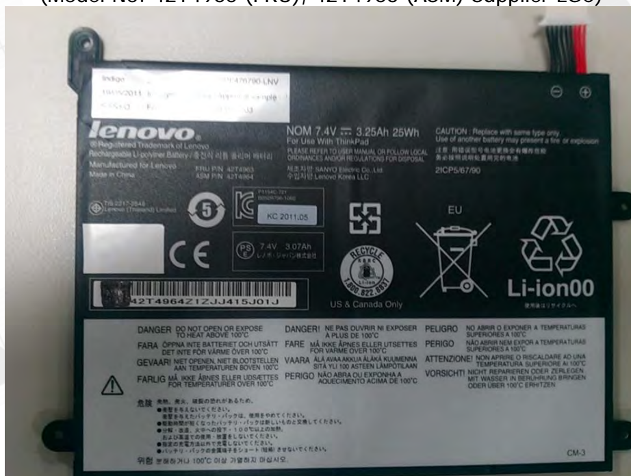
Fig.11 Front view of Battery (Model No: 42T4963 (FRU), 42T4964 (ASM), Supplier: Sanyo)
