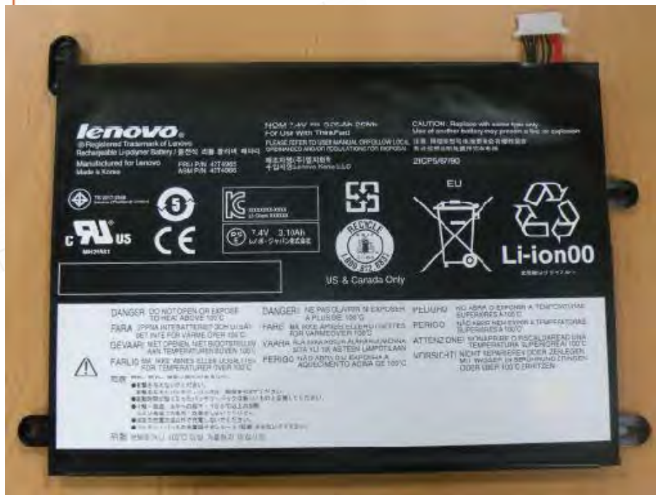
Fig.10 Front view of Battery (Model No: 42T4965 (FRU), 42T4966 (ASM) Supplier LGC)
