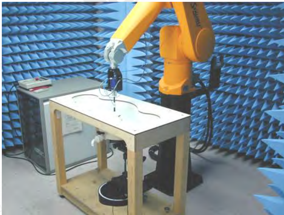
Fig.1 Photograph of the SAR measurement System
