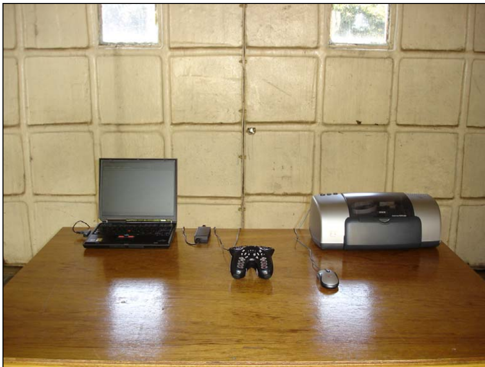
Photograph 2: Setup for Radiated Emissions
