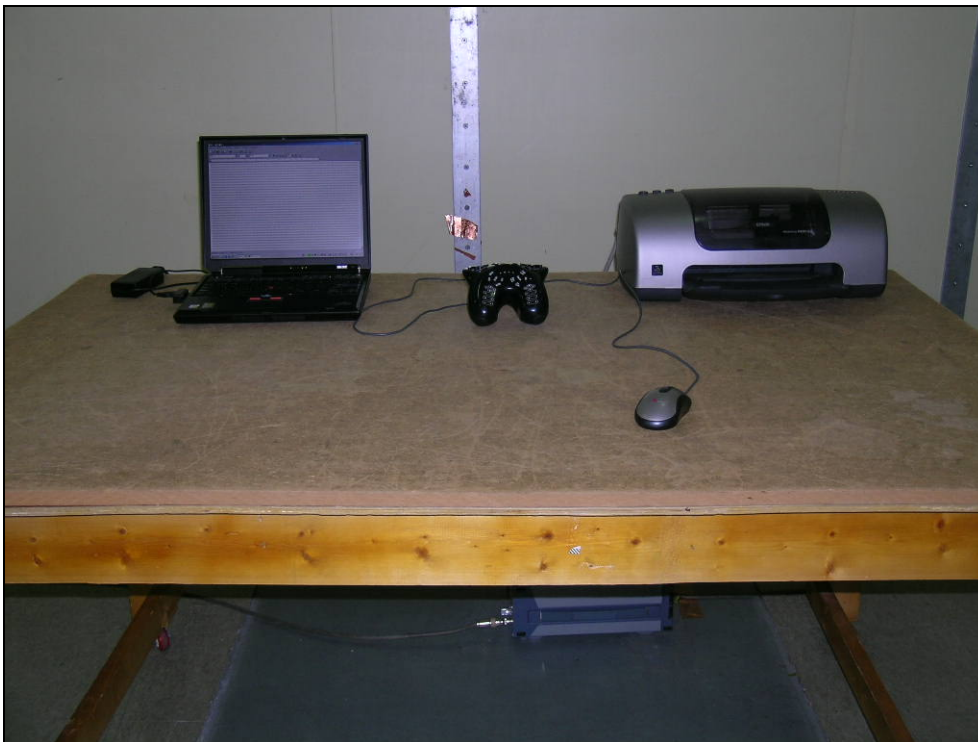
Photograph 1: Setup for Conducted Emissions
