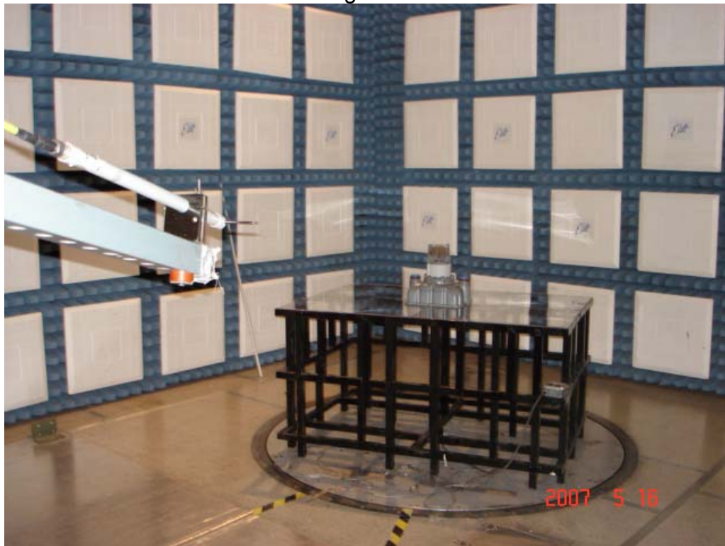
Test Set-up for Radiated Emissions, 911.65MHz to 921.25MHz Horizontal Polarization
