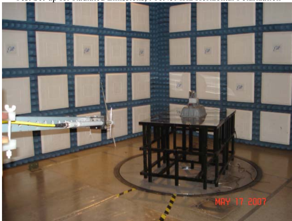
Test Set-up for Radiated Emissions, 916.45MHz Vertical Polarization
